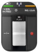
Slide switch: fast forward, play/record, stop, rewind (LFH3020)
