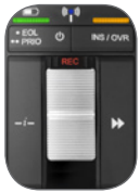
Slide switch: record, stop, play, rewind (LFH3010)
